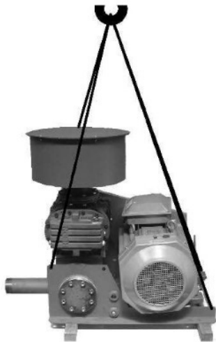
Figure 5 Lifting the unit without an enclosure fitted
