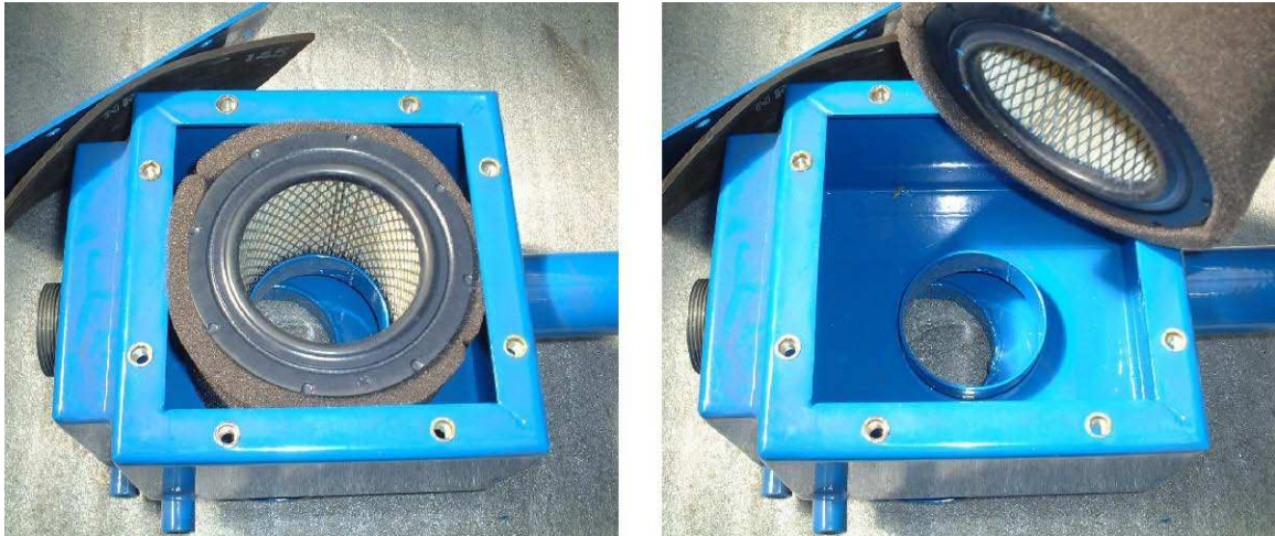
Figure 16 Exhauster filter cartridge replacement
