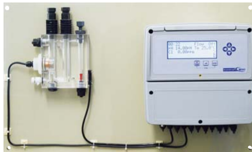
Kontrol 800 Panel version with transparent Modular Probe Holder PSS-Plexi
