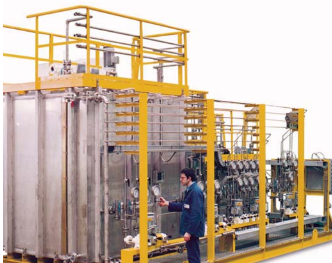
Corrosion inhibitor, Antifoam and Antiscaling Injection Package
