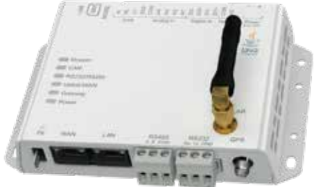
ChemitecWeb Instrument monitoring and set-up through HTTPS protocol via GPRS
