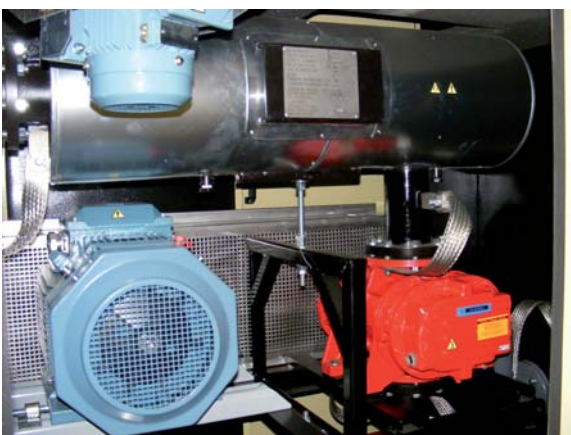
Package in version ATEX with acoustic enclosure
