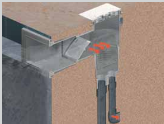
• Plastic floating weir with basket
