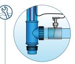
The amalgam version includes a flow switch that will turn off the lamp when the flow is too low. The UV-C amalgam lamp is less affected by temperature fluctuations in the water and generates a constant, powerful radiation. Amalgam UV-C light is known as being the most powerful UV-C light available on the UV-C market.
