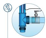
The amalgam version includes a flow switch that will turn off the lamp when the flow is too low. The UV-C amalgam lamp is less affected by temperature fluctuations in the water and generates a constant, powerful radiation. Amalgam UV-C light is known as being the most powerful UV-C light available on the UV-C market.
