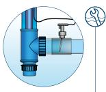
The Inox includes a flow switch that will turn off the lamp when the flow is too low. The Inox UV-C 130W includes an amalgam lamp. The UV-C amalgam lamp is less affected by temperature fluctuations in the water and generates a constant, powerful radiation. Amalgam UV-C light is known as being the most powerful UV-C light available on the UV-C market. The housing of the Inox UV-C is completely made of 316L stainless steel and is the driving disinfection force for (high-end) pools.
