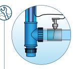
The amalgam version includes a flow switch that will turn off the lamp when the flow is too low. The UV-C amalgam lamp is less affected by temperature fluctuations in the water and generates a constant, powerful radiation. Amalgam UV-C light is known as being the most powerful UV-C light available on the UV-C market.
